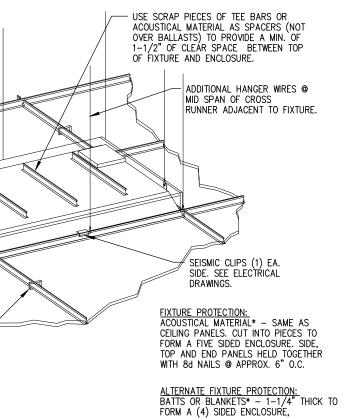
TRIANGULAR IN SECTION. LAP OVER ADJACENT PANELS 4". HELD TOGETHER W/ #18SWG GALV. STEEL WIRE. U.L. DESIGN #J201
