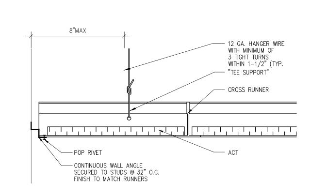
TYPICAL LAY-IN CEILING @ ATTACHED END Scale: 3" = 1'- 0"
